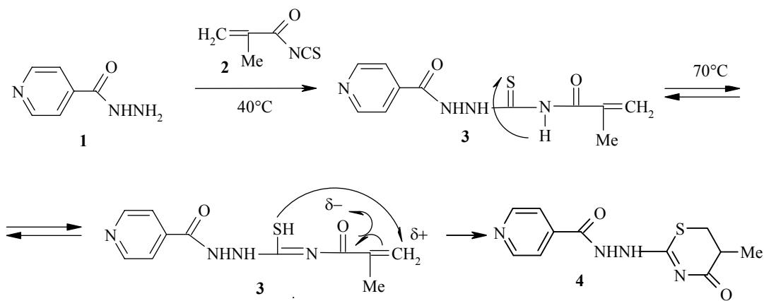
Compound **3** was formed at 30-40°C in 2-propanol or ethanol. On increasing the reaction time to 16 h and increasing the temperature of the reaction mixture to 70°C, the product of its intramolecular heterocyclization –  $\beta$ -N-(5-methyl-4-oxo-5,6-dihydro-4H-1,3-thiazin-2-yl)isonicotinohydrazide (**4**), formed by a scheme for the formation of 1,3-thiazine derivatives which has not previously been described in the literature.
